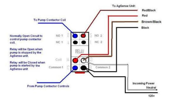
When "start" is sent to the unit from the web/cell, the pump control relay will turn on and stay on. When "stop" is sent to the unit from the web/cell, the pump control relay will turn off and stay off until started from the web/cell again.
